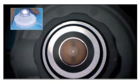
4) Make sure it is carefully centered on the chamber prior to placing the cover over the cornea to seal the chamber. Inflate the chamber with an air syringe to reverse the cornea, then close the valve to stabilize the chamber. Do not over-pressurize.
