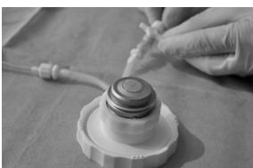
Precisely center the cornea on the stage and place the cover carefully in position (inserting the pin into the slot). Check that the graft is well centered. Seal the chamber by placing the white locking ring over the cover. Open the chamber stopcock at least three seconds. Then, close the chamber stopcock to maintain pressure of 90 mmHg. **Check the 2 stopcocks are closed.**
